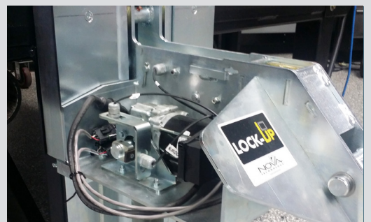
Sealed magnetic proximity sensors with direct drive gear motor
