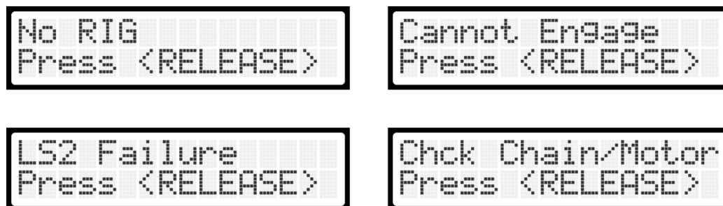
FIGURE 7.T—RESTRAINT LOCKING FAULTS
